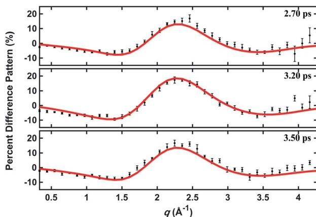
Fig. 5 Experimental and calculated percent difference scattering patterns at several representative delay time points. The experimental results (black dots) are adopted from ref. 14 with  $3\sigma$  error bars and scaled to 100% excitation. Calculated scattering patterns (red lines) are computed using the structural parameters determined with the present method, using the Wigner pool and a computed electronic correction term as described in the text.
