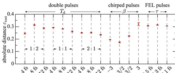
Fig. 2 Absolute distance error  $\varepsilon_{\text{test}}$  eqn (8d), of the different predicted spectra for test data: *double pulses* with time delay  $T_d$  and amplitude ratios  $A_1 : A_2$  as indicated, *chirped pulses* with chirp parameter  $\beta$ , and *partially coherent pulses* with coherence time  $\tau$ .
