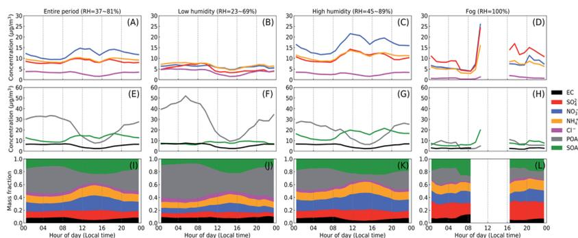
Fig. 3 Diel variations of the submicron aerosol (PM<sub>1</sub>) mass concentrations (A–H) and mass fractions (I–L) of the major components of submicron aerosols (PM<sub>1</sub>) averaged over the entire campaign and focus periods with different relative humidity (RH) conditions. The solid lines in (A–H) show the mean value of hourly averaged concentrations of each component. The displayed RH range relevant to each focus period is based on daily averaged data.
