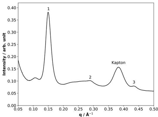
Fig. 1 The initial SAXS pattern of a  $73 \pm 2 \mu\text{m}$  thick film. Numbers indicate the lamellar phase Bragg peaks. The scattering peak from Kapton film on the X-ray detector is also labelled and was used as an internal standard.
