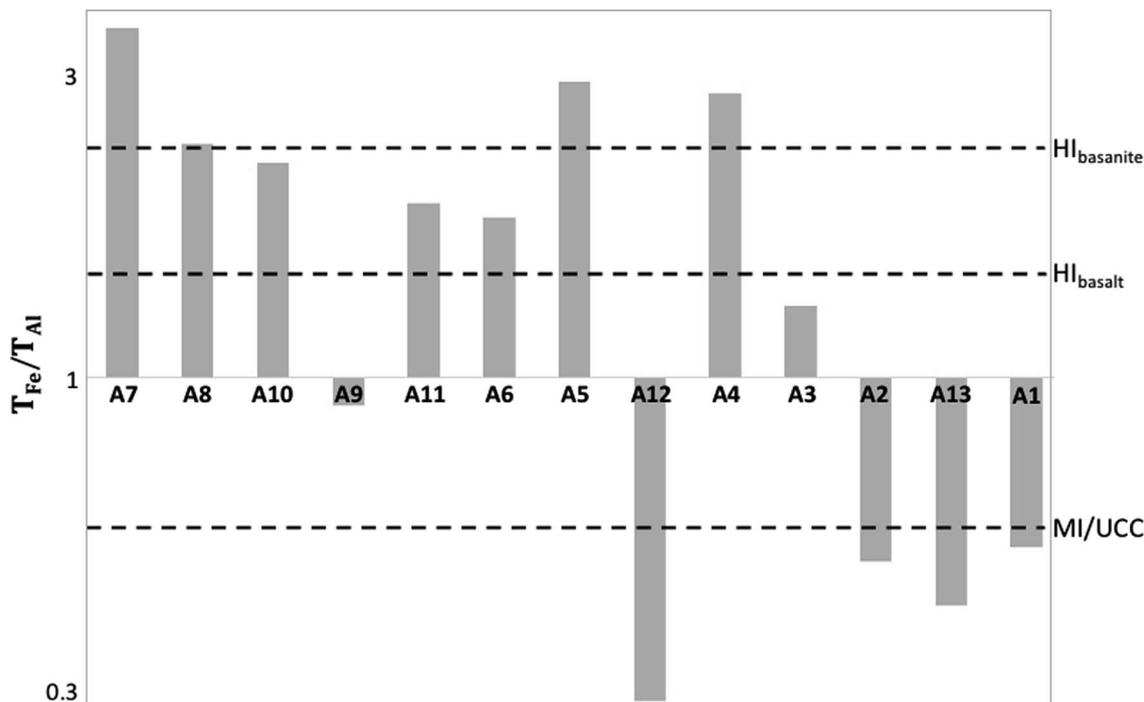
Fig. 1 Total concentration ratio of Fe-to-Al,  $T_{Fe}/T_{Al}$ , in aerosols collected during the HEOBI campaign. Horizontal dashed lines represent the same ratio measured in the averaged upper continental crust (UCC from McLennan *et al.*, (2001)<sup>24</sup>) and in rocks dredged near Heard Island (HI) and McDonald Island (MI) for comparison. A log scale view was chosen for better visualization of the different  $T_{Fe}/T_{Al}$  ratios between samples.
