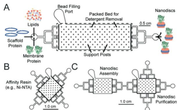
Fig. 7 Graphical representation of the microfluidic chips used in the formation (A) and purification (B) of lipid nanodiscs. The group show the facile connection of both modules to generate a bifunctional chip. Reproduced with permission from The Royal Society of Chemistry.<sup>100</sup>
