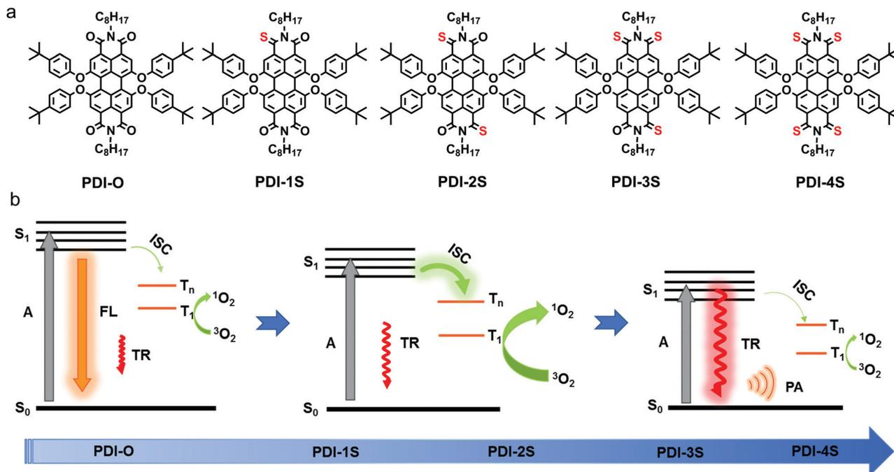
**Scheme 1** (a) Chemical structures of thionated PDIs, and (b) schematic illustration of manipulating phototheranostic effects through the controlling of thionation degree (A: absorption, FL: fluorescence, TR: thermal radiation, ISC: intersystem crossing, PA: photoacoustic).
