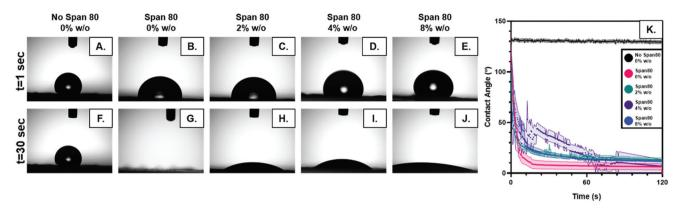
Fig. 5 (A-E) Contact angle of water on electrospun mesh with increasing internal phase and no Span 80 control at 1 second. (F-J) Contact angle of water at 30 seconds. (K) Plot of contact angle for each group over time.
