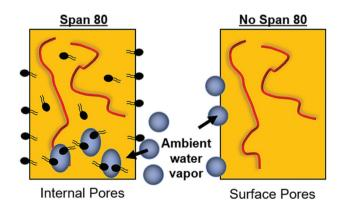
**Fig. 4** Ambient water interaction with fiber during electrospinning. In fibers with Span 80, water penetrates the core of the fiber. In fibers without Span 80, water droplets only condense on the fiber surface.
