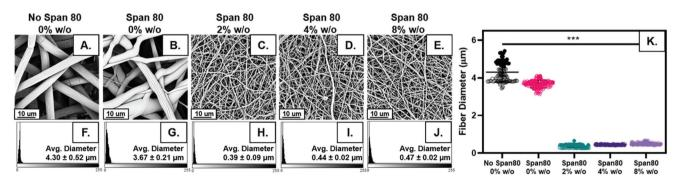
Fig. 2 (A-E) SEM micrographs of electrospun fibers with increasing internal phase volume fraction and control. (F-J) Representative histograms of fiber diameter distribution for increasing internal phase volume fraction and control. (K) Dot plot of fiber diameter for each group. Data points from the same mesh are indicated by closed, open, or x shapes in the circle. \*  $p \le 0.05$ ; \*\*  $p \le 0.01$ ; \*\*\*  $p \le 0.001$ .
