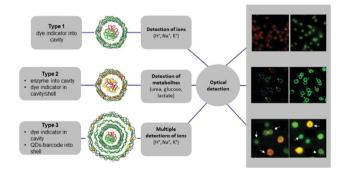
Fig. 9 Different types of LbL-based sensors. Type 1 (typically for ion detection): ion-sensitive indicators reside in the cavity. Type 2 (typically for metabolite detection): metabolite-degrading enzymes and indicator dyes are present inside the cavity, or indicator dyes are incorporated in the outer shell. Type 3 (for multiplex ion detection): Type 1 with QD-based barcode placed in the outermost shell. Modified from ref. 8 with permission of Elsevier B.V.
