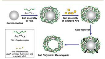
**Fig. 8** Schematic representation of LbL assembly. PEM capsules are produced by LbL adsorption of oppositely charged polyelectrolytes (green and gray) onto spherical charged spheres, followed by dissolution of sacrificial templates. During LbL coating, various charged elements can be incorporated within the multilayers to add functionality to the capsules. Adapted from ref. 8 with permission of Elsevier B.V.
