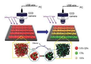
$\begin{tabular}{ll} Scheme 1 & Principle of the C/CdTe-GOx aerogel microsensor to detect glucose. \end{tabular}$
