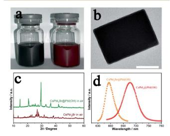
Fig. 4 CsPbl<sub>2</sub>Br prepared by our solution method. (a) Photographs of CsPbl3@Pbl(OH) and CsPbl2Br@Pbl(OH) prepared in solution. (b) TEM image of CsPbl2Br@Pbl(OH). Scale bar: 150 nm. (c) PXRD patterns of CsPbl<sub>2</sub>Br@Pbl(OH) and  $\gamma$ -CsPbl<sub>2</sub>Br in air, showing degradation for the latter, which does not have a PbI(OH) protective shell. (d) Photoluminescence spectra of CsPbI3@PbI(OH) and CsPbI2Br@PbI(OH).
