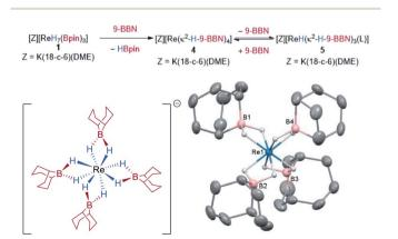
Scheme 4 Synthesis of 4 from 1 by borane exchange and the solidstate structure of 4. For clarity, the cation [K(DME)(18-c-6)]<sup>+</sup> and all hydrogen atoms except for the Re hydrides are omitted; displacement ellipsoids are drawn at 50% probability.
