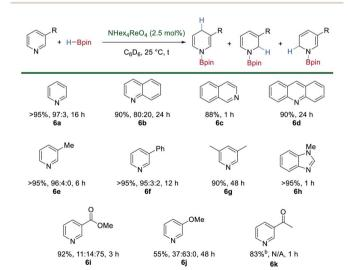
Scheme 5 Catalytic hydroboration of N-heteroaromatics using  $[N(hexyl)_4][ReO_4]$  as a pre-catalyst and HBpin. For **6k** reduction is observed exclusively at the carbonyl when 1 equivalent of HBpin is used.
