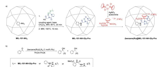
Fig. 2 Synthesis and catalytic application of (benzene)Ru@MIL-101-NH-Gly-Pro. (a) Post-synthetic peptide grafting and metalation of the Al-MIL-101-NH<sub>2</sub> with the chiral benzene ruthenium prolinamide complex; (b) acetophenone asymmetric transfer hydrogenation catalyzed by benzene ruthenium species combined with MOF macroligand or molecular ligands,  $L^1$  and  $L^2$  (see Section 4 in ESI†).
