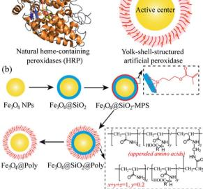
Scheme 1 (a) Representative structures of natural heme-containing peroxidase (left) and yolk-shell-structured artificial peroxidase (right). (b) Preparation procedures of the yolk-shell-structured artificial peroxidase.
