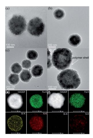
Fig. 1 TEM images of (a) Fe<sub>3</sub>O<sub>4</sub> NPs, (b) Fe<sub>3</sub>O<sub>4</sub>@SiO<sub>2</sub>, (c) Fe<sub>3</sub>O<sub>4</sub>@- $SiO_2@Poly(L-Trp)$ , and (d)  $yolk-shell Fe_3O_4@Poly(L-Trp)$ . (e) and (f) show the TEM elemental mapping images of Fe<sub>3</sub>O<sub>4</sub>@SiO<sub>2</sub>@Poly(L-Trp) and yolk-shell  $Fe_3O_4@Poly(L-Trp)$ , respectively.
