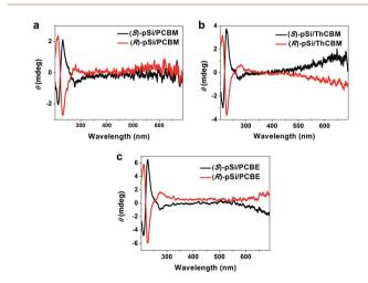
Fig. 6 CD spectra of (a) (S or R)-pSi/PCBM, (b) (S or R)-pSi/ThCBM, and (c) (S or R)-pSi/PCBE films. The films were prepared by spin-coating the blend solutions of the chiral surface modifier (1.5 mg mL $^{-1}$ ) and fullerene derivative (10 mg mL $^{-1}$ ). After spin-coating, the films were annealed at 150 °C for 30 min.
