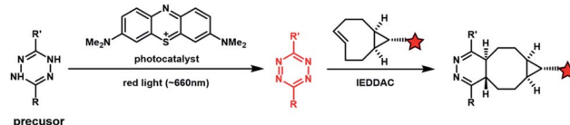
Fig. 4 Photocatalytic activation of the IEDDAC reaction.
