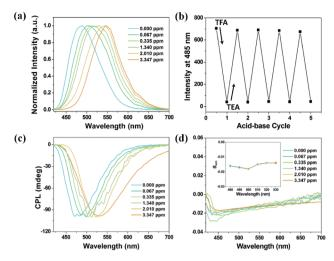
Fig. 5 (a) Normalized fluorescence of xerogel films treated with increasing amounts of TFA (0, 0.067, 0.335, 1.340, 2.010, and 3.347 ppm) for 10 s at 298 K ( $\lambda_{\rm ex}=410$  nm). (b) The reversible switch of emission intensity of xerogel films at 485 nm by alternating TFA and TEA stimuli. (c) CPL spectra and (d)  $g_{\rm lum}$  of xerogel films upon protonation ( $\lambda_{\rm ex}=370$  nm).
