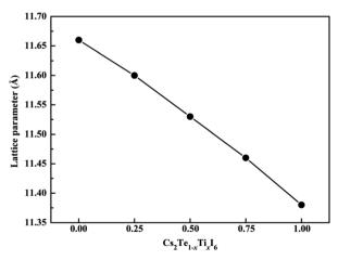
Fig. 2 The lattice constants of the  $Cs_2Te_{1-x}Ti_xI_6$  solid solutions.
