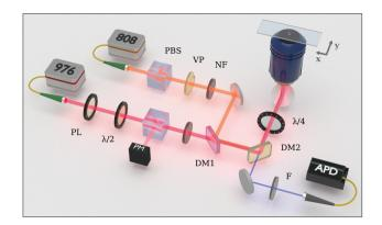
Fig. 1 Schematic of the confocal microscope system, where PBS is a polarising beam splitter, VP a vortex plate, NF a neutral density filter, PL is a polariser,  $\lambda/2$  a half-wave plate, PM a power meter, DM1 and DM2 respectively a long-pass and short-pass dichroic mirror,  $\lambda/4$  a quarterwave plate, F a blue narrow-band filter, and APD an avalanche photodiode.
