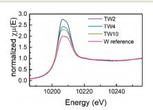
Fig. 5 W  $\mbox{L}_3\mbox{-edge}$  XANES spectra of three W-doped  $\mbox{TiO}_2$  and W-reference samples.
