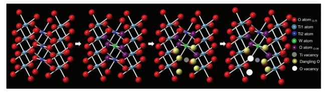
Fig. 7 A schematic illustration of W-doping induced structural change to TiO<sub>2</sub>.
