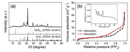
Fig. 2 (a) XRD pattern and (b) N<sub>2</sub> adsorption/desorption isotherms and pore size distribution curve (inset) of the MoS<sub>2</sub>@SnS heterostructure.
