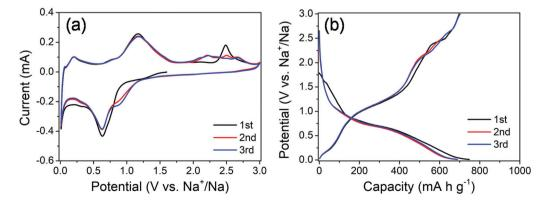
Fig. 5 (a) CV curves of the MoS<sub>2</sub>@SnS heterostructure at a scan rate of 0.1 mV s<sup>-1</sup> and (b) galvanostatic charge/discharge profiles of the MoS<sub>2</sub>@SnS heterostructure at a current density of 0.1 A  $g^{-1}$ .
