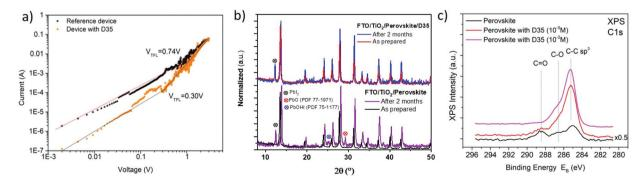
Fig. 8 The I-V curves for electron-only devices with and without D35 (a); XRPD patterns of fresh and aged perovskite films with and without D35 treatment (b); and XPS measurements for perovskite films without and with D35 in two different concentrations ( $10^{-5}$  M and  $10^{-2}$  M) (c).
