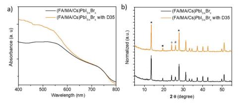
Fig. 2 UV-vis absorption spectra (a) and XRPD patterns (b) of mixed perovskite films with and without D35 treatment. Symbols "\*", "o" and "#" represent the perovskite, FTO and TiO<sub>2</sub> peaks, respectively.
