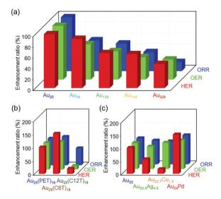
Fig. 7 Enhancement ratio of the HER, OER, and ORR activities for gold clusters with different (a) sizes, (b) ligands, and (c) metal substitutions compared with the case for  $[Au_{25}(PET)_{18}]^0$ .
