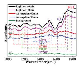
Fig. 7 In situ FTIR spectra of C-ZNNS60: (a) in the absence of CO<sub>2</sub> and H<sub>2</sub>O in the dark, after adsorption of CO<sub>2</sub> and H<sub>2</sub>O for (b) 30 min and (c) 60 min in the dark, and under light irradiation for (d) 30 min and (e) 60 min.
