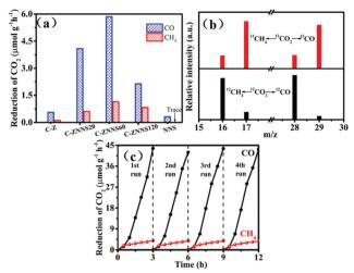
Fig. 6 (a) Photocatalytic CO<sub>2</sub> reduction performances of all samples. (b) CO and CH<sub>4</sub> mass spectra of C-ZNNS60. (c) Cyclic CO<sub>2</sub> reduction curves for CO and CH<sub>4</sub> yield (350 W, NaHCO<sub>3</sub> = 1 mmol).
