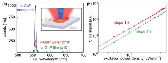
Fig. 2 (a) Spectral SHG response at a fundamental wavelength of 1120 nm and 10.2 µW mm<sup>-2</sup> average pump power for the c-GaP wafer (red), a-GaP film (green) and a single a-GaP nanopatch (blue). Inset: Sketch of the SHG measurement of a GaP nanopatch on glass substrate. (b) Power dependence for the c-GaP wafer and a-GaP film at double logarithmic scale. The dashed lines represent a fitting to a linear model resulting in the indicated slopes.
