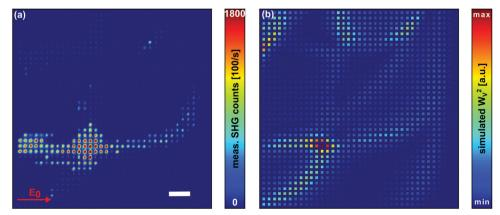
Fig. 4 (a) SHG measurement of the entire nanopatch array from Fig. 2a. The fundamental wavelength is 1120 nm with an average excitation power of 25.5  $\mu$ W mm<sup>-2</sup>. The red arrow indicates the pump polarization. Scale bar: 10  $\mu$ m. (b) Numerical simulation of the square of the electric energy ( $W_V^2$ ) for the array in (a). Each square represents the respective patch with dimensions corresponding to this position.
