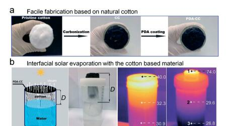
Fig. 12 Low-cost cotton based solar evaporator. (a) The rapid fabrication of light absorbing cotton. (b) The oil lamp inspired solar evaporator exhibits an obvious interfacial heating ability.<sup>70</sup>
