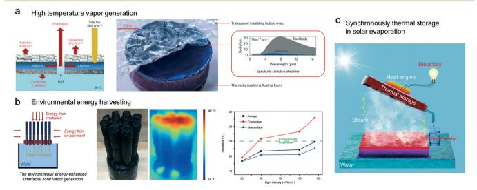
Fig. 10 Innovative solar evaporators with heat managing design. (a) The evaporator with multi-level high insulation for high temperature vapor generation.<sup>59</sup> (b) Smart design for harvesting environmental energy through a wetted side wall. (c) Harnessing the heat of vapor by the water collector for electricity generation.<sup>66</sup>
