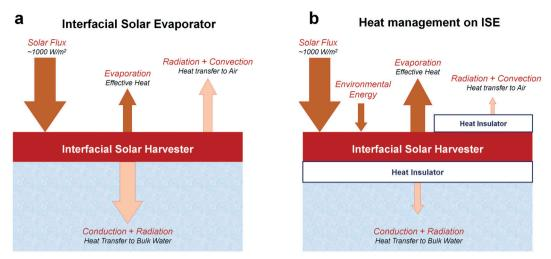
Fig. 9 The heat transfer during the interfacial solar evaporation (ISE). (a) The conventional evaporator and (b) the novel evaporation system with precise heat management.
