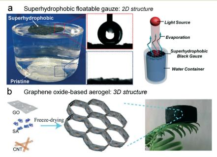
Fig. 5 Intrinsically floatable solar evaporators. (a) The carbon black-based, self-cleaning, superhydrophobic gauze for efficient solar evaporation at the air-water interface.<sup>45</sup> (b) The graphene oxide-based aerogel with ultralow density for solar steam generation.<sup>47</sup>
