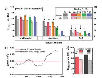
Fig. 6 (A) Solid Pt and (Ru<sub>v</sub>Ti<sub>1-v</sub>)O<sub>2</sub>-coated Ti electrodes in various water-methanol solvent systems, (B) graph showing a constant and simulated wind-energy current density profile and (C) comparison of the efficiency and selectivity for the respective electrolysis using RuO2coated Ti electrodes. 61 Reprinted from ref. 61, Copyright (2018), with permission from the American Chemical Society.
