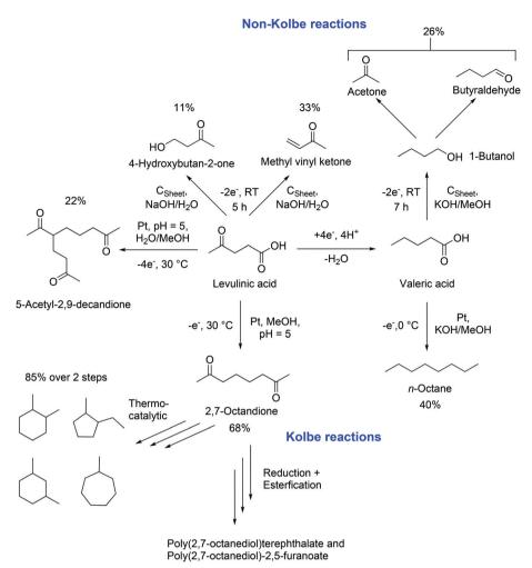
Scheme 4 Synthesis possibilities starting from levulinic acid LA and valeric acid VA, based on the research results of Schröder 18,19 Yuan 96 and Mascal. 104 The reaction conditions were selected according to the maximal achieved yield.
