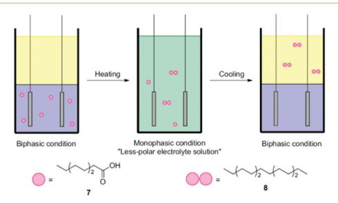
Fig. 4 Illustration of the coupling of octanoic acid using a thermomorphic system. Reprinted from ref. 74, Copyright (2012), with permission from Elsevier.
