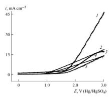
**Fig. 5** Voltammograms of the electrooxidation of a mixture of 10-undecylenic and acetic acid and sodium acetate in EtOH on different electrodes: (1) Ir, (2) pyrographite, (3) glassy carbon SU-2000, (4) graphite, (5) Pt.<sup>70</sup> Reprinted from ref. 70, Copyright (2013), with permission from Springer Nature.
