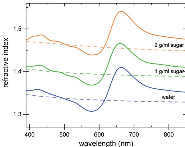
Fig. 4 Refractive index variation of 100 mM Brilliant Blue dissolved in water (bottom curve), 1 g mL<sup>-1</sup> sugar solution (middle curve) and 2 g mL<sup>-1</sup> sugar solution (top curve). The dashed lines show the dye-free reference.
