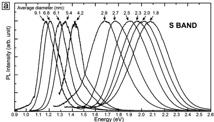
Fig. 12 S-band 300 K PL from the various-sized nanocrystals of Fig. 11.<sup>188</sup> Adapted with permission from Y. Yu, G. Fan, A. Fermi, R. Mazzaro, V. Morandi, P. Ceroni, D. M. Smilgies and B. A. Korgel, *J. Phys. Chem. C*, 2017, **121**, 23240–23248. Copyright 2007 American Chemical Society.
