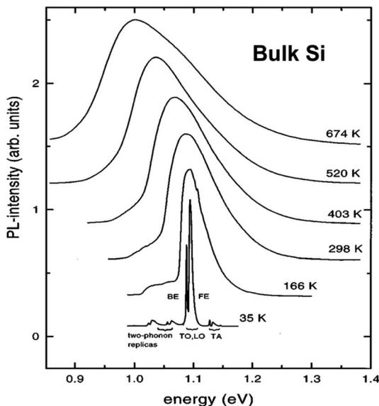
Fig. 2 Normalized interband PL from bulk Si at 35–674 K.<sup>29</sup> BE stands for bound exciton, FE for free exciton (see text). Reprinted with permission from V. Alex, S. Finkbeiner and J. Weber, *J. Appl. Phys.*, 1996, 79, 6943. Copyright AIP Publishing.
