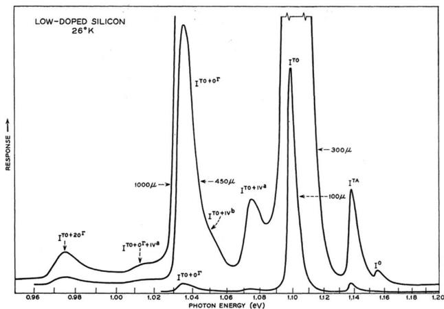
Fig. 3 Intrinsic free exciton PL from high purity silicon at 26 K.<sup>16</sup> The LO and TO phonon components are not resolved. Reprinted with permission from P. J. Dean, J. R. Haynes and W. F. Flood, *Phys. Rev.*, **161**, 711–729. Copyright the American Physical Society, 1967.
