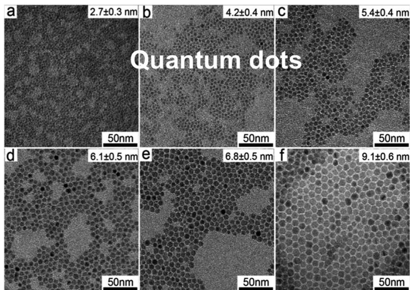
Fig. 11 S-band photoluminescent silicon nanocrystals of controllable size.<sup>188</sup> Adapted with permission from Y. Yu, G. Fan, A. Fermi, R. Mazzaro, V. Morandi, P. Ceroni, D. M. Smilgies and B. A. Korgel, *J. Phys. Chem. C*, 2017, **121**, 23240–23248. Copyright 2007 American Chemical Society.
