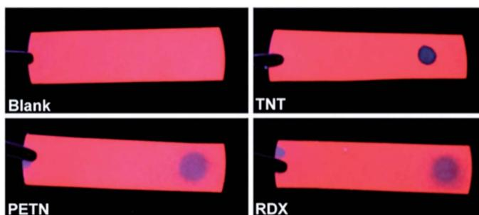
Fig. 18 S-band sensing of explosives.<sup>314</sup> Reproduced with permission from C. M. Gonzalez, M. Iqbal, M. Dasog, D. G. Piercey, R. Lockwood, T. M. Kipotke and J. G. C. Veinot, *Nanoscale*, 2014. Copyright Royal Society of Chemistry.
