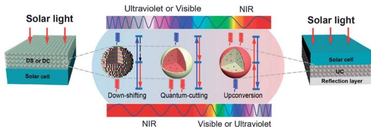
Fig. 20 Classes of spectral converters.<sup>413</sup> Reproduced with permission from C. X. Huang, S. Han, W. Huang and X. Liu, *Chem. Soc. Rev.*, 2013, **42**, 173–201. Copyright Royal Society of Chemistry.
