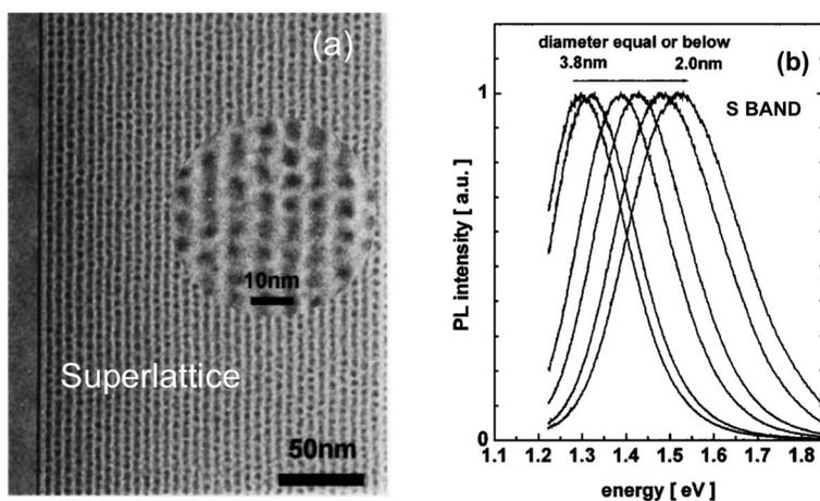
Fig. 9 Superlattice-based nanocrystals and their S-band photoluminescence.<sup>171</sup> Reprinted and adapted with permission from M. Zacharias, J. Heitmann, R. Scholz, U. Kahler, M. Schmidt and J. Blasing, *Appl. Phys. Lett.*, 2002, **80**(4), 661–663. Copyright AIP Publishing.
