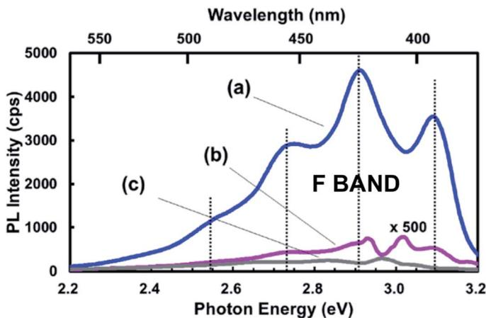
Fig. 16 Photoluminescence of adsorbed fluorescent organic contaminants on silicon nanoparticles.<sup>268</sup> Adapted with permission from T. Matsumoto, M. Maeda and H. Kobayashi, *Nanoscale Res. Lett.*, 2016, 11(7), available via an open access CC-BY license.
