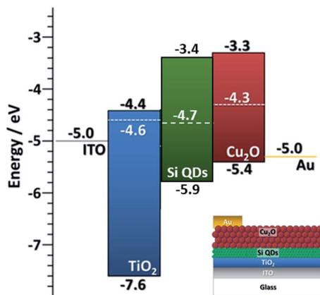
Fig. 6 Non-equilibrated band diagram for the PV device based on Si QDs as active layers, Cu<sub>2</sub>O QDs as an electron blocking layer, a TiO<sub>2</sub> film hole blocking layer and corresponding contacts. Inset: diagram of the layer structure of the device.
