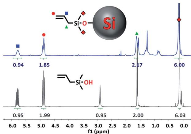
Fig. 3 <sup>1</sup>H NMR spectrum of 1-Si NPs (top) and pure unbound 1 (bottom) in CDCl<sub>3</sub>.
