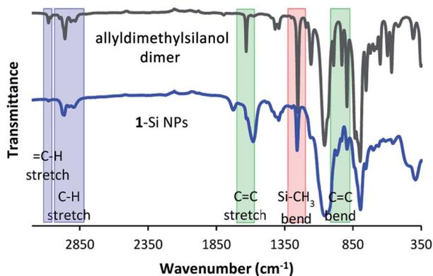
Fig. 4 ATR-IR spectra of **1**<sub>2</sub> and 1-Si NPs. Several notable peaks are highlighted.
