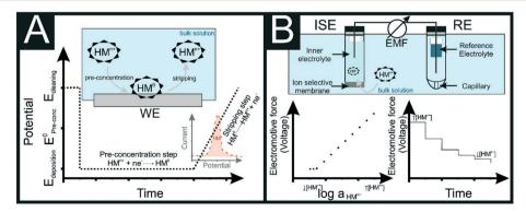
Fig. 3 Schematic diagram of a potentiostatic (anodic stripping voltammetry; A) and a potentiometric (ion-selective electrode (ISE); B) method respectively.
