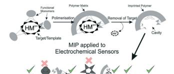
**Fig. 4** Schematic representing MIPs applied to electrochemical sensor platforms.
