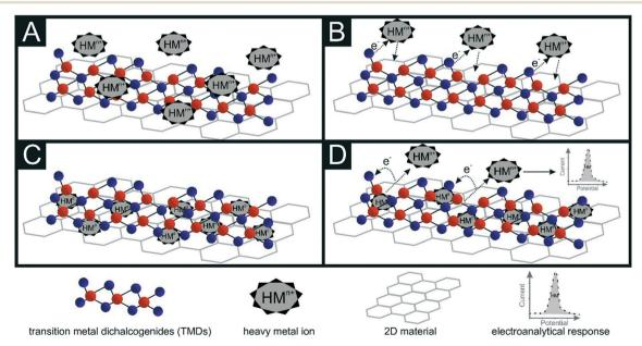
Fig. 5 Schematic representing the electrochemical steps when TMDS are used within an electrochemical sensor: pre-measurement (A), deposition potential application (B), pre-accumulation step (C) and stripping step (D).
