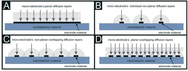
Fig. 6 Schematic represensing the catergories of diffusion profiles at different micro-electrode array configurations. Planar diffusion layers at macro-electrodes (A), individual non-planar diffusion layers at micro-electrodes (B), non-overlapping diffusion layers at micro-electrodes (C) and planar overlapping diffusion layers at micro-electrodes (D).
