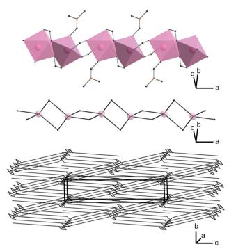
Fig. 4 Octahedrally coordinated cadmium( $\pi$ ) in 2 forming chains along the a axis (top), its transformed  $4^2$ -net (middle) and the resulting final dmd net-type (bottom).
