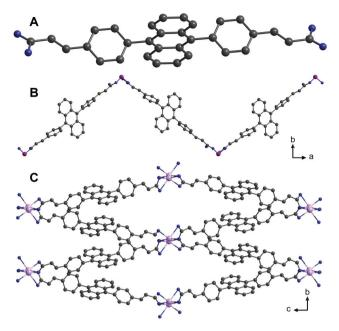
Fig. 1 Solid-state structures of (A)  $H_2L$ , (B) one-dimensional coordination polymer  $\{[Zn(L)(DMF)_2]\}_n$  (1) and (C) a three-dimensional metalorganic framework  $\{[Cd(L)(DMF)]\cdot DMF\}_n$  (2) based on 4,4'-(9,10-anthracenediyl)dicinnamic acid  $(H_2L)$ . Solvent molecules and hydrogen atoms were omitted for clarity. Colour code: C, black; O, blue; Zn, purple; Cd: pink.
