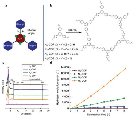
Fig. 9 (a) A tunable triphenylarene structure. (b) Formation of  $N_x$ -COFs based on hydrazine and  $N_x$ -aldehydes. (c) PXRD patterns of  $N_x$ -COFs compared with the simulated pattern calculated for the representative  $N_3$ -COF. (d)  $H_2$  production monitored over 8 h using  $N_x$ -COFs as a photocatalyst in the presence of triethanolamine as a sacrificial electron donor. Reproduced with permission from ref. 102. Copyright 2015 Macmillan Publishers Limited.
