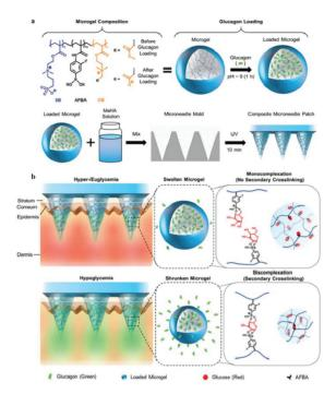
Fig. 13 (a) Schematic illustration of the glucose-sensitive composite microneedle patch based on zwitterionic nanogel. (b) Schematic of hypoglycemia-triggered delivery of glucagon. Reprinted with permission from ref. 147 Copyright 2019, John Wiley and Sons.
