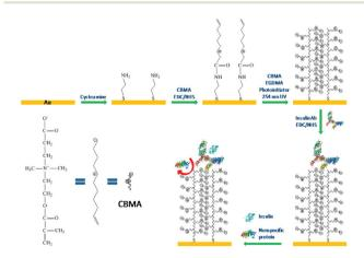
**Fig. 12** Schematic illustration of the fabrication of insulin receptive interface and its antifouling and selective insulin-binding properties. Reprinted with permission from ref. 143 Copyright 2013, American Chemical Society.
