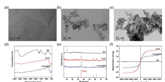
Fig. 1 NP characterization. TEM images of (a) GO, (b)  $Fe_3O_4$ , and (c)  $Fe_3O_4$ @GO MNCs. (d) FTIR spectra of GO,  $Fe_3O_4$ , and  $Fe_3O_4$ @GO MNCs. (e) XRD patterns of GO,  $Fe_3O_4$ , and  $Fe_3O_4$ @GO MNCs (the red lines at the bottom mark the reference pattern of  $Fe_3O_4$  from the JCPDS database, card number 19-0629). (f) Room-temperature hysteresis curves of GO,  $Fe_3O_4$ , and  $Fe_3O_4$ @GO MNCs.
