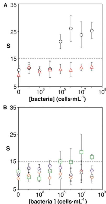
**Fig. 3** Calibration plots representing the colorimetric signal *S* with respect to the concentration of pathogens. (A) *E. coli* (black dots) and *S. viridans* (red triangles); (B) *E. faecalis* (green squares); *K. pneumoniae* (purple dots); *P. mirabilis* (orange diamonds), *E. cloacae* (grey triangles) (semi-logarithmic scale). Dotted lines show the signal above 3 times the standard deviation of the *E. coli* blank. Error bars are the standard deviation ( $n = 3$ ).
