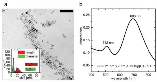
Fig. 1 Characterization of the gold nanorods. (a) TEM image of gold nanorods. The image analysis for 320 particles shows a mean length of  $21 \pm 5$  nm, a mean diameter of  $7 \pm 2$  nm, and a mean aspect ratio of 3.16 (scale bar: 100 nm). (b) UV-Vis spectrum of the same gold nanorod sample after PEGylation. The longitudinal localized surface plasmon resonance (I-lspr) was measured to be 690 nm.
