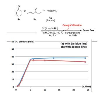
Fig. 1 Hot filtration test.
