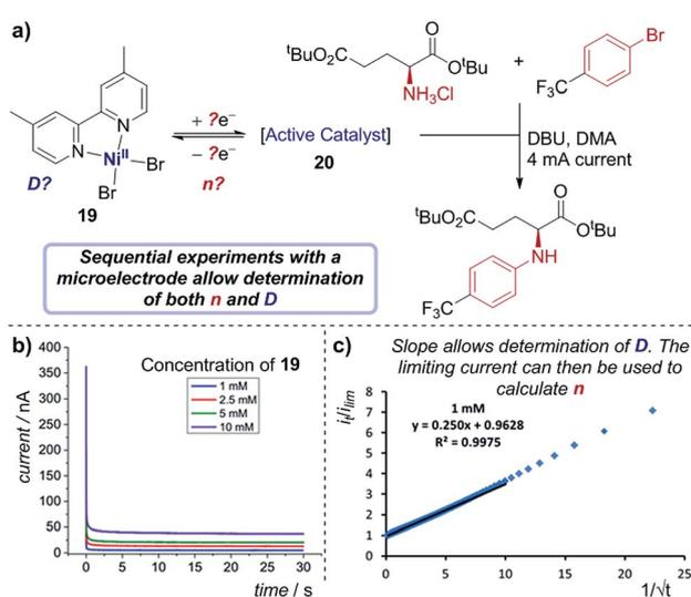
Fig. 20 (a) Determination of both the diffusion coefficient and number of electrons transferred in the reduction of **19**, by the groups of Baran, Minter, Neurock and White. The current response upon application of a potential step is measured (b), and the slope of the plot in (c) allows determination of the diffusion coefficient. Positive current represents reduction. (b and c) Adapted with permission from ref. 39c. Copyright 2019 American Chemical Society.
