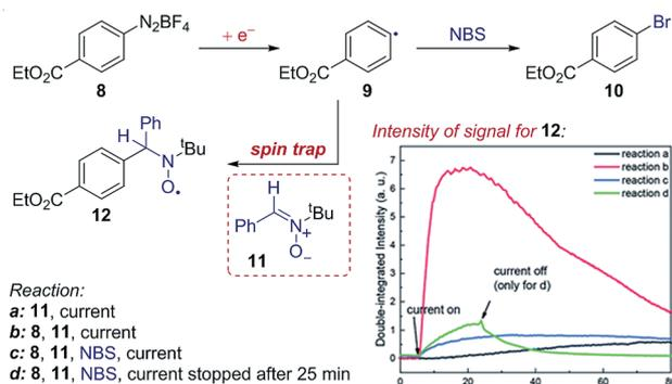
Fig. 15 EPR spectroelectrochemistry provides evidence for the formation of radical **9** following electrochemical reduction, and the subsequent reaction with *N*-bromosuccinimide (NBS), reported by Mo and co-workers. The formation of radical **9** is measured by the EPR signal of the long-lived radical **12** afforded by spin-trapping. Adapted with permission from ref. 50. Copyright 2018 The Royal Society of Chemistry.
