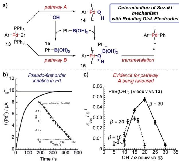
Fig. 16 RDE experiments provide evidence for a palladium-hydroxyl species as a catalytic intermediate in the Suzuki cross-coupling reaction, reported by Amatore *et al.* For inset in (b),  $x$  is the fractional conversion to Pd(0). (a) Adapted with permission from ref. 58. Copyright 2013 John Wiley and Sons. (b and c) Adapted with permission from ref. 57. Copyright 2011 John Wiley and Sons.
