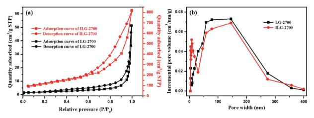
Fig. 5  $N_2$  adsorption–desorption isotherms (a) and pore size distribution (b) of LG-2700 and ILG-2700.
