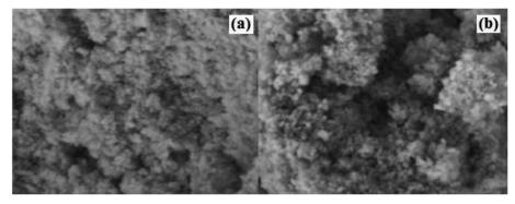
Fig. 5 The FE-SEM images of Pd@MTiO<sub>2</sub> material at high (a) and low (b) resolutions
