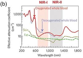
Fig. 1 Visible, NIR-I, and NIR-II windows. (a) Reduced scattering coefficients  $(\mu_s)$  of various biological tissues as a function of wavelength. (b) Effective attenuation coefficients of fat, skin, and blood as a function of wavelength. (a and b) Reproduced from ref. 17 and 18 with permission from the Nature Publishing Group, Copyright 2017 and 2009, respectively.
