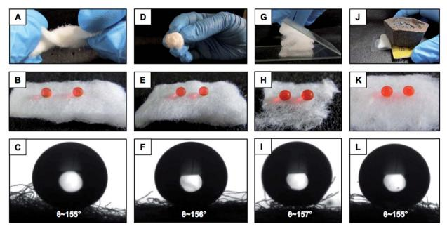
Fig. 3 Digital images (A, B, D and E) and contact angle images (C and F) depicting various physical manipulations, i.e., twisting (A–C) and winding (D–F) of the BSA derived superhydrophobic cotton. Digital images (H and K) and contact angle images (I and L) showing the impact of different abrasive physical durability tests—adhesive tape test (G) and sand paper abrasion test (J)—on the protein derived superhydrophobicity.
