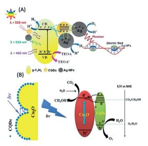
Fig. 10 Use of glucose-derived QDs for (A) the generation of  $H_2$  gas and (B) conversion of  $CO_2$  to methanol. (A) has been adapted/reproduced from ref. 161 with permission from John Wiley and Sons and (B) from ref. 162 with permission from Elsevier.
