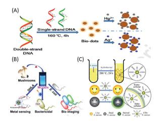
Fig. 5 Use of (A) nucleic acid (DNA), (B) fungus (mushroom) and (C) bacteria (S. aureus or E. coli) as a carbon sources to synthesize biomolecule-derived QDs. (A) has been adapted/reproduced from ref. 93 with permission from Elsevier, (B) from ref. 95 with permission from Elsevier, and (C) from ref. 97 with permission from The Royal Society of Chemistry.
