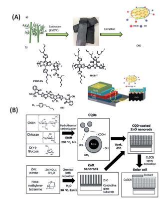
Fig. 9 Use of (A) bamboo- and (B) chitin-, chitosan- and glucosederived QDs for the fabrication of solar cells. (A) has been adapted/ reproduced from ref. 152 with permission from John Wiley and Sons and (B) from ref. 153 with permission from John Wiley and Sons.
