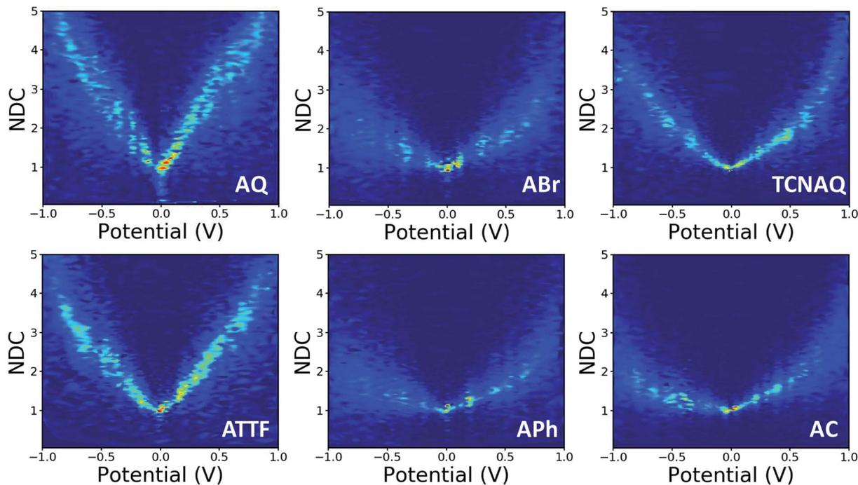
Fig. 5 Normalized differential conductance heatmaps for Au<sup>Mica</sup>/SAM//EGaIn junctions comprising AQ, ABr, TCNAQ, ATTF, APh, and AC.
