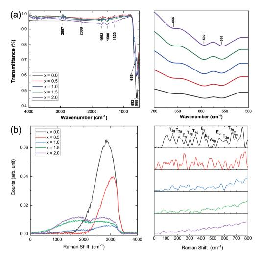
Fig. 3 (a) Infrared spectra and (b) Raman spectra of all the Ce<sup>3+</sup>-substituted YIG samples.
