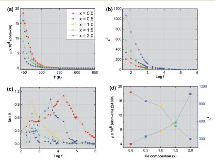
Fig. 8 (a) Variation of electrical resistivity ' $\rho$ ' as a function of temperature 'T', (b) variation of dielectric constant ' $\varepsilon$ ' as a function of logarithm of frequency 'log f', (c) variation in dielectric loss tangent 'tan  $\delta$ ' as a function of logarithm of frequency 'log f' and (d) variation of electrical resistivity ' $\rho$ ' measured at 450 K and dielectric constant ' $\varepsilon$ ' as a function of Ce composition.
