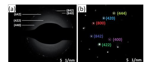
Fig. 6 SAED patterns of (a) polycrystalline YIG, x = 0.0, and (b) preferred (100) oriented single-crystalline Ce-YIG, x = 2.0.
