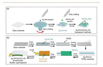
Scheme 1 Schematic of the fabrication of (a) the Ag NW/Ni(OH)<sub>2</sub> NS TE and (b) the all-solid-state flexible supercapacitor.
