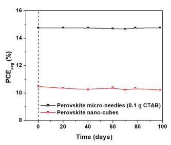
Fig. 6 Long-term stability test of un-encapsulated devices based on MAPbl<sub>3</sub> micro-needles and perovskite nano-cubes stored in dry air.
