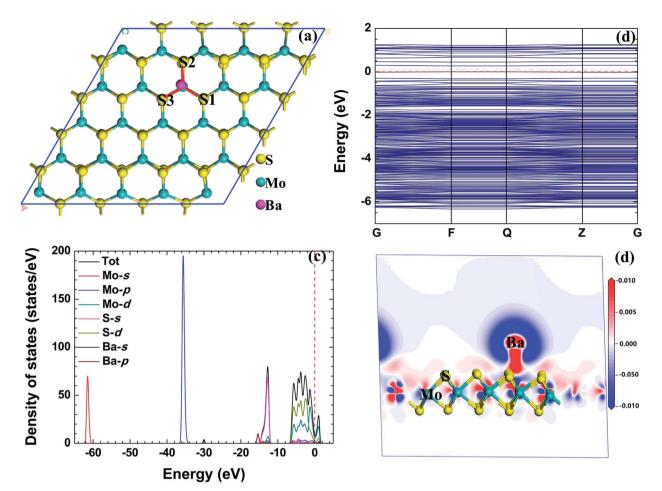
Fig. 5 The relaxed configuration, band structure (from -10 eV to 5 eV), density of states, and electron density difference of the radionuclide Ba adsorbed on monolayer MoS2 with the initial configuration B.
