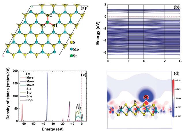
Fig. 4 The relaxed configuration, band structure (from -10 eV to 5 eV), density of states, and electron density difference of the radionuclide Sr on monolayer MoS<sub>2</sub>.
