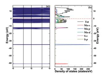
Fig. 2 The band structure (a) and density of states (b) of monolayer MoS<sub>2</sub>, and the red dashed lines stand for the Fermi level.
