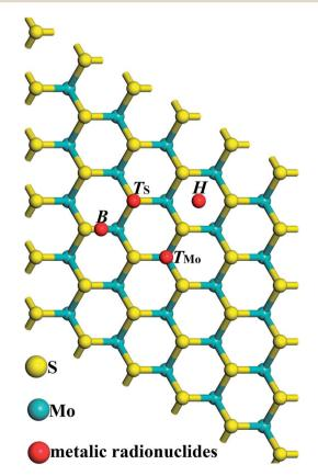
Fig. 1 Schematic diagram of the possible adsorption sites of a metallic radionuclide on monolayer MoS2, and glaucous, yellow, and red balls represent Mo atoms, S atoms, and metallic radionuclides, respectively.
